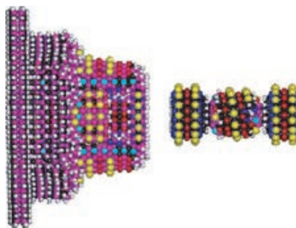
Fig. 6. Side views of a 6165-atom neon gas pump/motor. 132 Image courtesy of K. Eric Drexler. © Institute for Molecular Manufacturing (www.imm.org).
