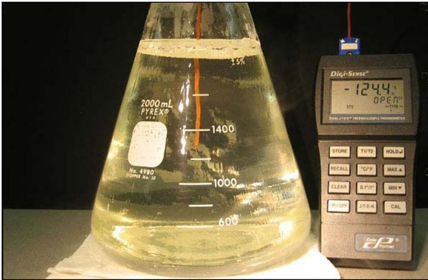
**Figure 3. Two liters (5 pounds) of M22 solution cooled at 0.14°C/minute (18 hours) until vitrified at a temperature of -124°C.**
