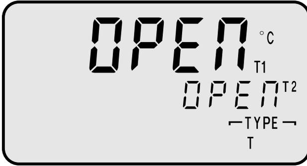
*This display shows that both ports are open, and no thermocouple probes have been connected. If you see this, check the connections.*
