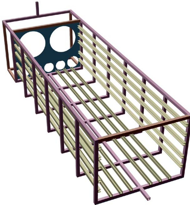
Figure 19-9. The design from Figure 19-8 with channel-section aluminum strips added to act as heat sinks. Color has been added to enable easier identification of the parts, and has no other significance.
