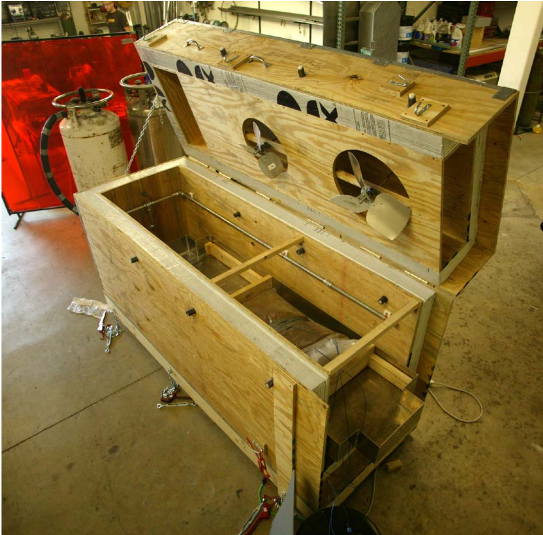
Figure 19-5. Prototype rapid cooldown box designed by Charles Platt and Gary Battiato at Suspended Animation in 2005. The fans were driven by motors mounted externally on the lid of the box. Sheets of foam board were used as insulation.
