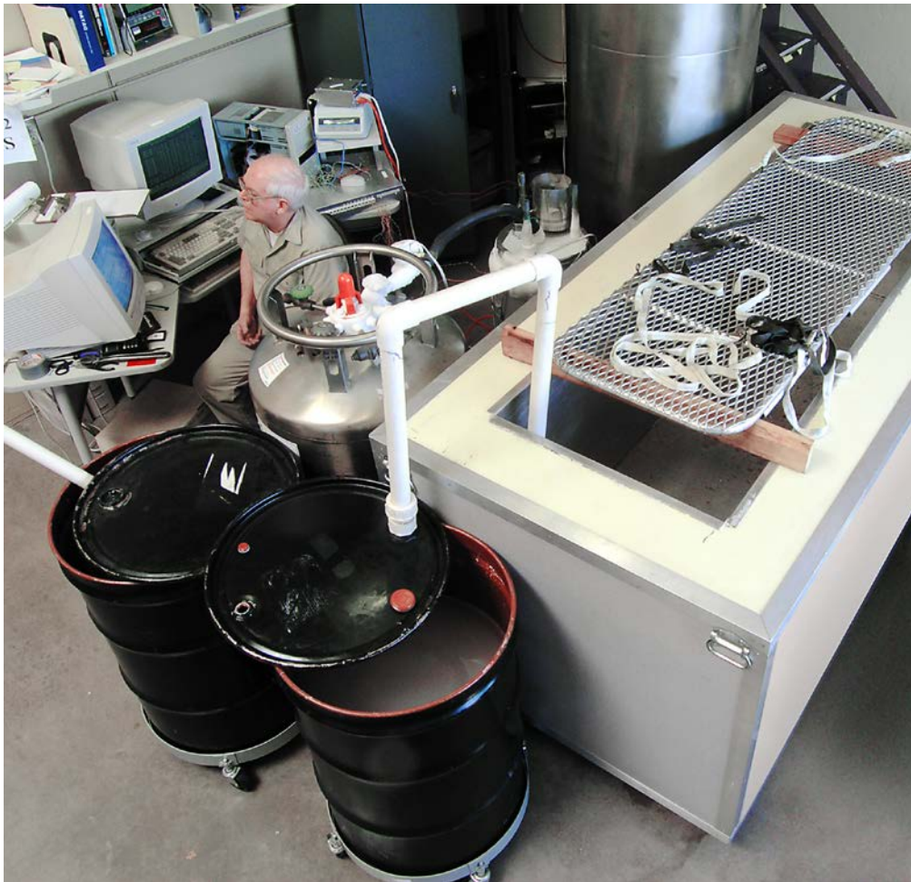
Figure 19-1. Hugh Hixon sitting beside the silicone-oil cooldown box that he designed. It is now used for cooling patients in rapidly circulating liquid nitrogen vapor.
