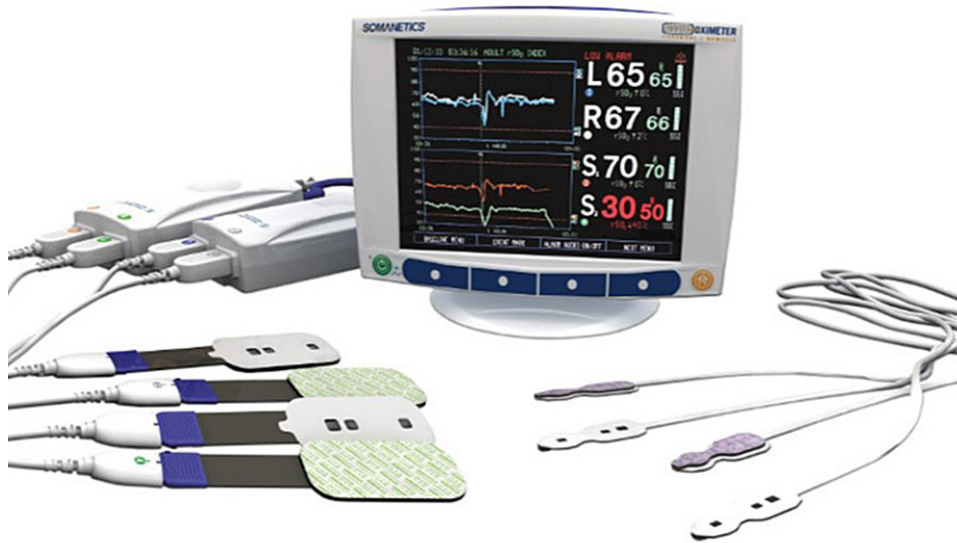
Figure 14-7. Four-channel version of the INVOS 5100C Cerebral/Somatic Oximeter showing adult-size and child-size sensors.
