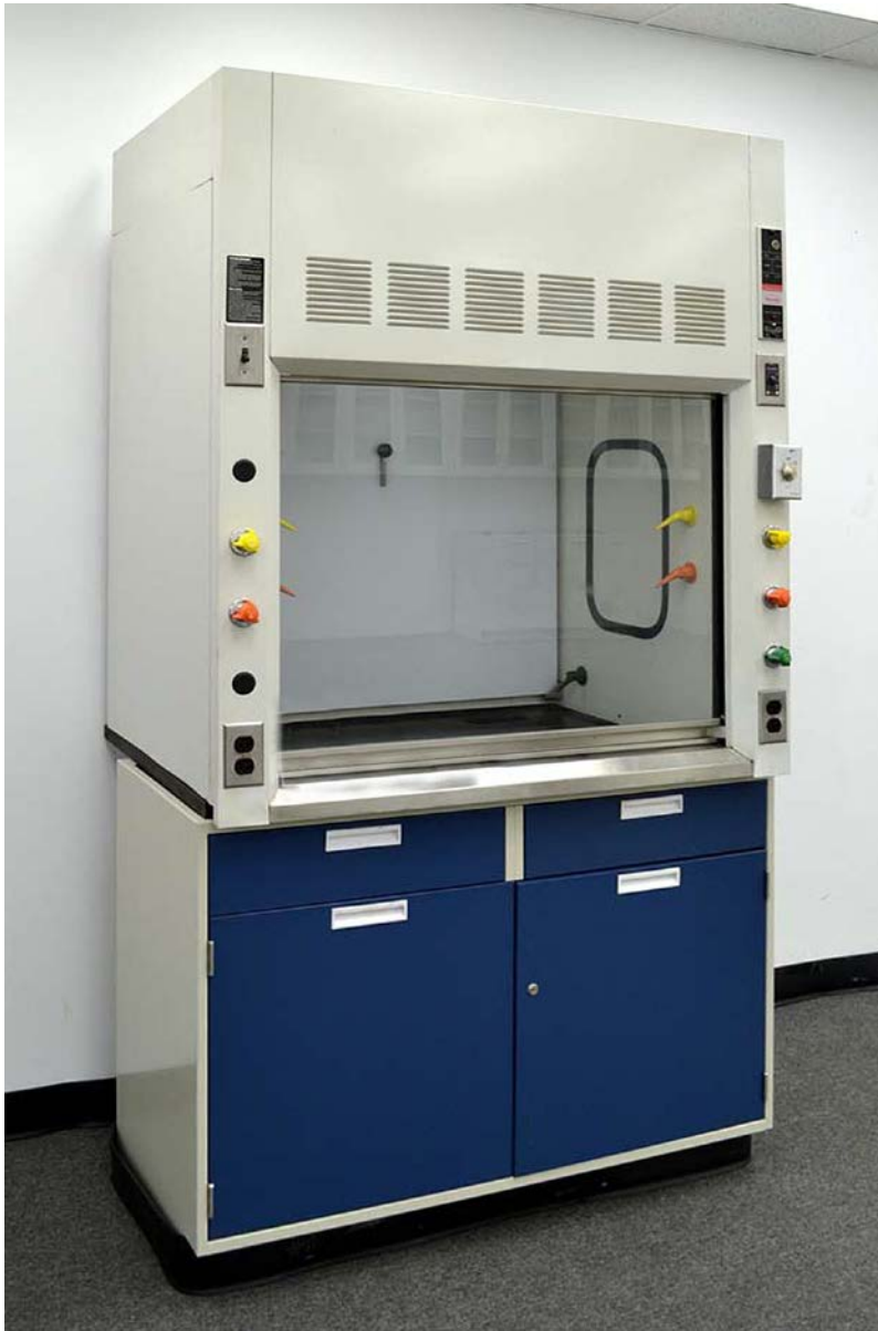
Figure 8-1. Fume Hood for protection against toxic chemicals and gases.
