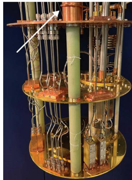
*NIST physicists measured and controlled a superconducting quantum bit (qubit) using light-conducting fiber (indicated by white arrow) instead of metal electrical cables like the 14 shown here inside a cryostat. By using fiber, researchers could potentially pack a million qubits into a quantum computer rather than just a few thousand. Credit: F. Lecocq/NIST*
