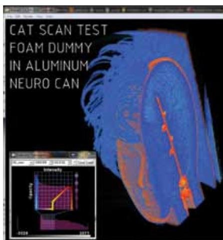
*Figure 1: Cross section of dummy head showing expanding foam in blue and center support in orange. CLUT manipulation tool (inset) which allowed this image to appear from the data. Less dense materials (foam and hair in blue) to the left side with more dense plastics to the right.*
