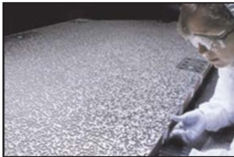
This coded aperture helps Swift spot gamma ray bursts —NASA photo.
