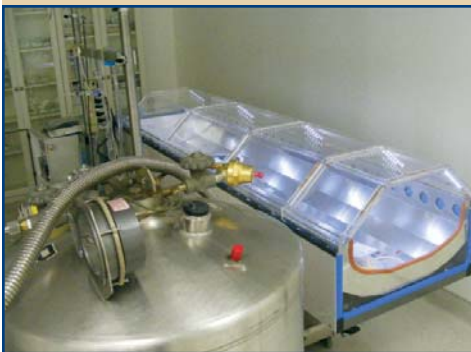
The patient enclosure cools the patient during surgery using nitrogen vapor and a cooling stage for the base.
