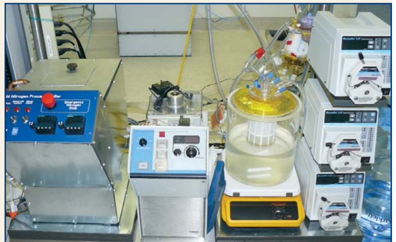
Equipment for automation of the perfusion process includes (from left to right): a chiller, a main pump, a mixing reservoir and pumps for addition and removal of cryoprotectants.
