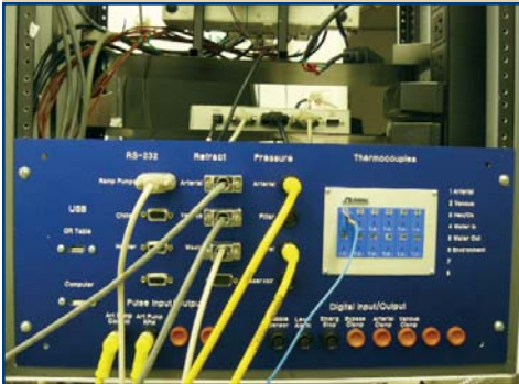
This panel shows some of the many connections the computer will automatically monitor and control during the perfusion process.
