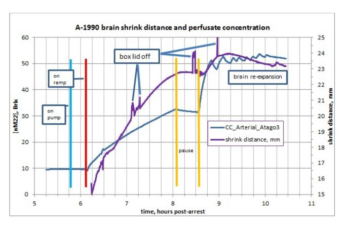
Note: Using a laser, the Brain Retraction Detection Device (BRDD) measures the contraction and expansion of the brain surface directly below a burr hole during cryoprotection. The output from the device is calibrated to derive a standardized reading in millimeters.
